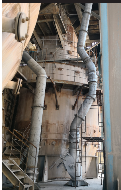
Preheated raw meal chute and exhaust gas duct
